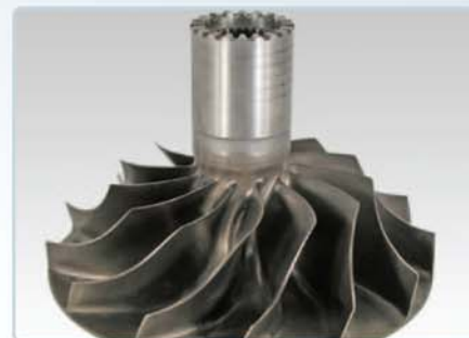
Impeller repaired by LENS 850-R System
