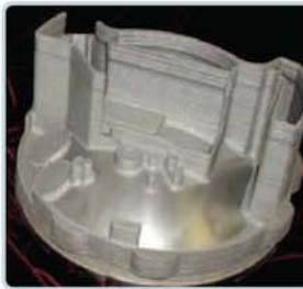
Defense Housing Fabricated by LENS System
