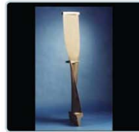
Compressor Blade Repaired by LENS System
