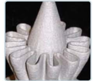
Exhaust Duct Fabricated by LENS System
