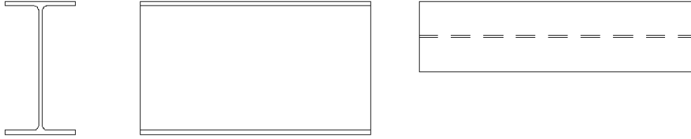
Figure 5-22: The W12x30 shape in section, elevation and plan views.
